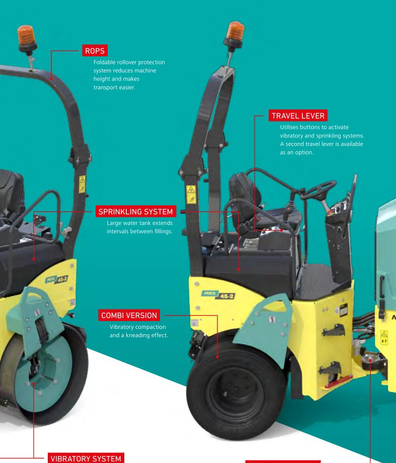
Great combination of high performance output and maintenance-free vibratory system make the machine more
