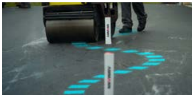
AWR 65-S Walk-Behind Roller with 15° steering angle
