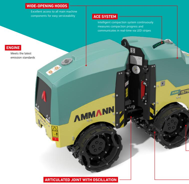
Connects the front and rear frame and ensures balanced weight distribution and permanent ground contact
